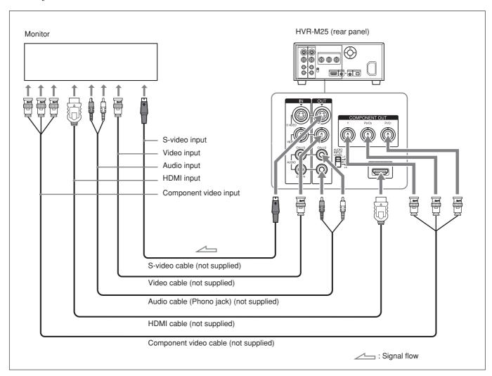
When an HDMI cable is used for connection, Audio cable connection is not necessary.
